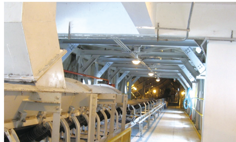
Total length: 2881m Belt width: 650mm, 800mm, 1000mm, 1200mm Transporting material: process material, bulk urea, finished product packing bag Installed power: 5.5~132kw Capacity: 100~600t/h Production date: December 2011
